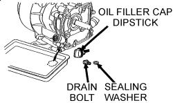
Figure 19. Engine Oil (Draining)
